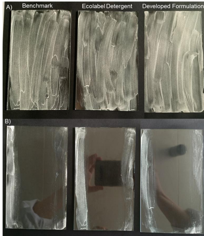
Figure D.1 - Performance test of glass cleaner using the cream gel as soil. Each glass tile corresponds to the benchmark, ecolabel certified detergent and the developed detergent, respectively. A) Appearance of the tiles at the beginning of the test. B) Appearance of the tiles at the end of the test.
