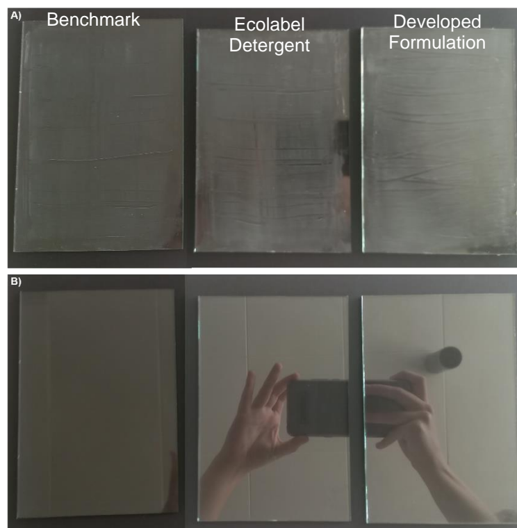
Figure 22 - Performance test of glass cleaner, using soap as soil. Each glass tile corresponds to the benchmark, ecolabel certified detergent and the developed detergent, respectively. A) Appearance of the tiles at the beginning of the test, B) Appearance of the tiles at the end of the test.
