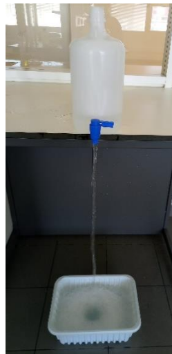
Figure 7 - Set up for hand dishwashing performance test
